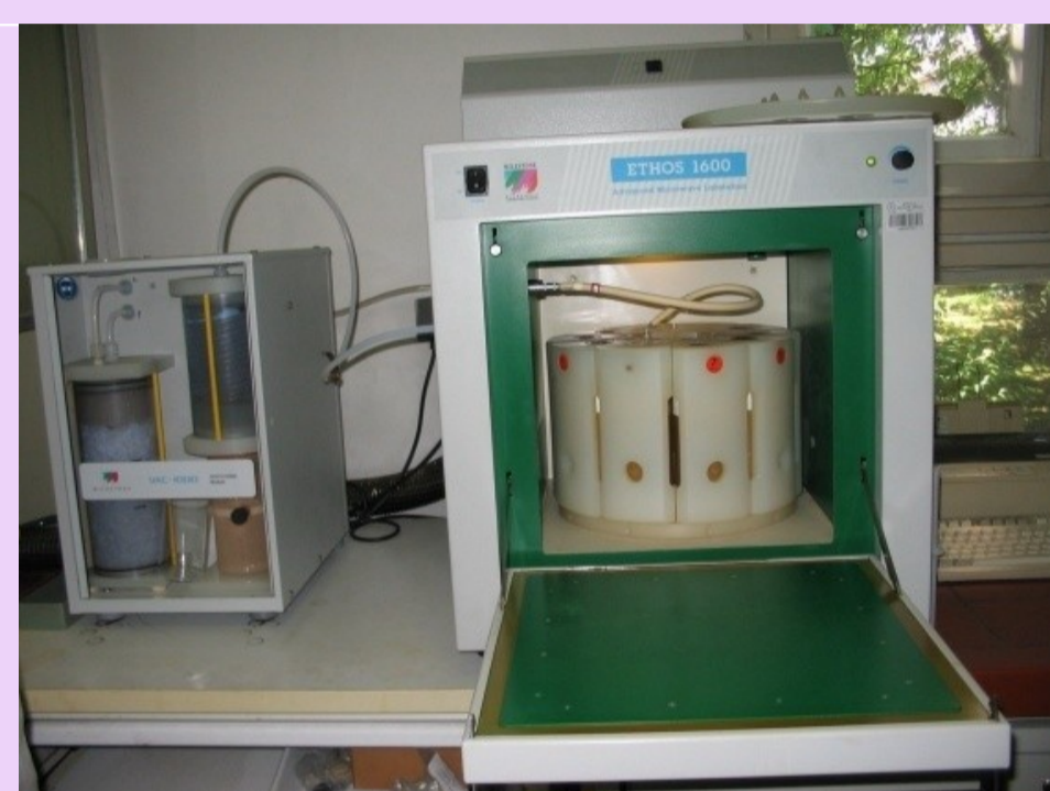
Sample preparation by microwave digestion of the Institute of Public Health in Ljubljana
