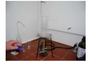
Pre-treatment of potatoes with a wet-oxidative acid mineralization
